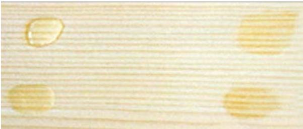
**Figure 3:** Unprotected board
