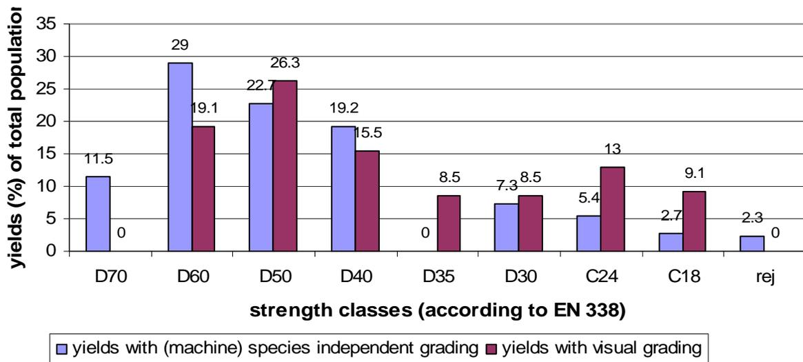
Figure 2. Comparison of grading yields for (machine) species independent grading with visual grading
