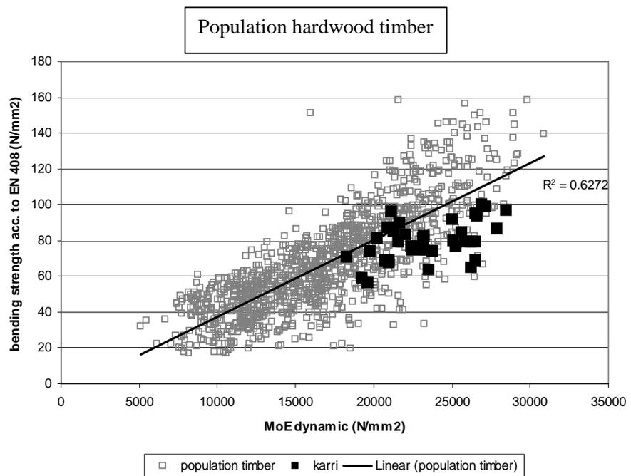
Figure 1. Test results for Karri and for all hardwood species together of the destructive bending strength according to EN 408 plotted against the dynamic modulus of elasticity
