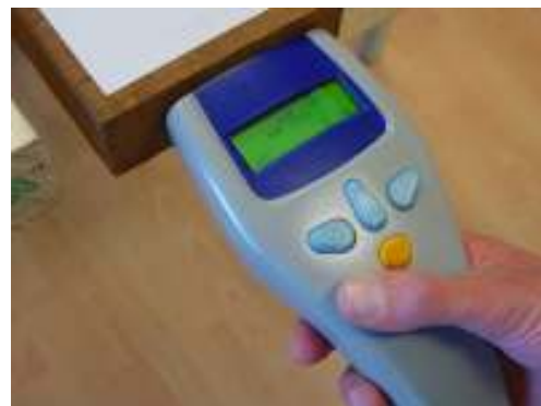
Figure 4 The Timber Grader MTG. An automatic hammer and sensor are integrated in the front that is placed on the end of the timber beam
